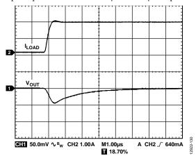
Figure 31. Output Transient Response,  $C_{OUT} = 10 \mu F$
