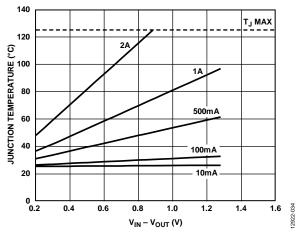
Figure 34. 6400 mm<sup>2</sup> of PCB Copper,  $T_A = 25$ °C
