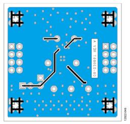
Figure 46. Typical Board Layout, Bottom Side
