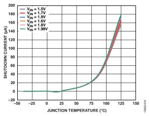
Figure 10. Shutdown Current vs. Junction Temperature at Various Input Voltages (V<sub>IN</sub>)
