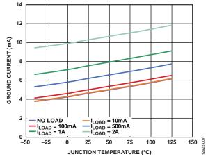
Figure 7. Ground Current vs. Junction Temperature
