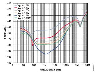
Figure 20. Power Supply Rejection Ratio (PSRR) vs. Frequency for Various  $V_{IN}$ ,  $V_{OUT} = 1.3 V$ , Load Current = 2 A
