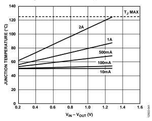
Figure 41. 500 mm<sup>2</sup> of PCB Copper,  $T_B = 50$  °C
