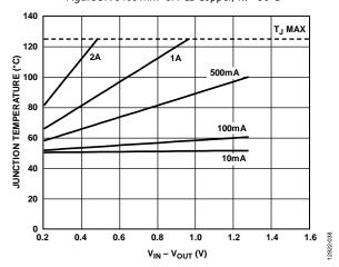
Figure 38. 500 mm<sup>2</sup> of PCB Copper,  $T_A = 50$ °C
