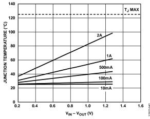
Figure 42. 1000 mm<sup>2</sup> of PCB Copper,  $T_B = 25$ °C
