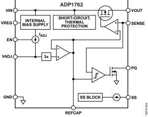
Figure 24. Functional Block Diagram, Adjustable Output
