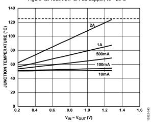
Figure 43. 1000 mm<sup>2</sup> of PCB Copper,  $T_B = 50$ °C
