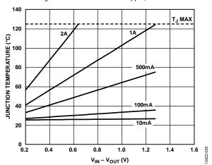
Figure 35. 500 mm<sup>2</sup> of PCB Copper,  $T_A = 25$ °C
