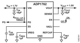
Figure 1. Fixed Output Operation
