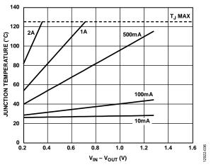
Figure 36. 25 mm<sup>2</sup> of PCB Copper,  $T_A = 25$ °C
