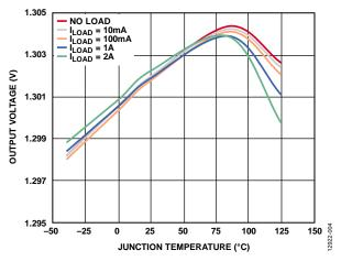
Figure 4. Output Voltage (V<sub>OUT</sub>) vs. Junction Temperature
