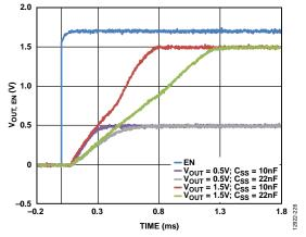
Figure 26. Adjustable V<sub>OUT</sub> Ramp-Up with External Soft Start Capacitor (V<sub>OUT, EN</sub>) vs. Time
