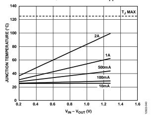
Figure 40. 500 mm<sup>2</sup> of PCB Copper,  $T_B = 25$ °C
