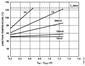
Figure 37. 6400 mm<sup>2</sup> of PCB Copper,  $T_A = 50^{\circ}\text{C}$
