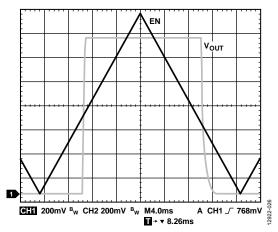
Figure 27. Typical EN Pin Operation
