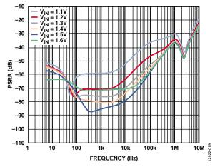
Figure 19. Power Supply Rejection Ratio (PSRR) vs. Frequency for Various  $V_{\text{IN}}$ ,  $V_{\text{OUT}} = 0.9 \, \text{V}$ , Load Current = 2 A
