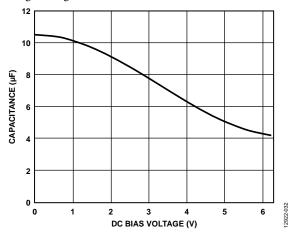
Figure 33. Capacitance vs. DC Bias Voltage
