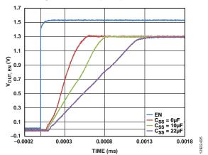
$\textit{Figure 25. Fixed V}_{\textit{OUT}} \textit{Ramp-Up with External Soft Start Capacitor (V}_{\textit{OUT,EN}} \textit{) vs. Time} \\$
