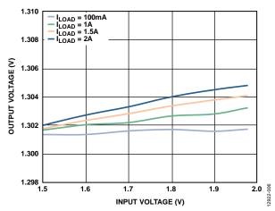
Figure 6. Output Voltage vs. Input Voltage
