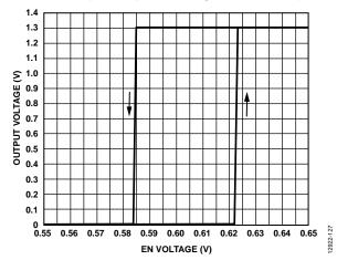
Figure 28. Output Voltage vs. Typical EN Pin Voltage,  $V_{OUT} = 1.3 \text{ V}$
