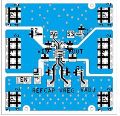
Figure 45. Typical Board Layout, Top Side
