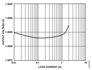
Figure 5. Output Voltage (Vout) vs. Load Current
