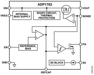
Figure 23. Functional Block Diagram, Fixed Output
