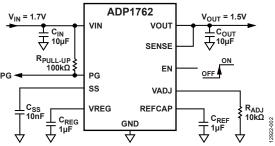
Figure 2. Adjustable Output Operation
