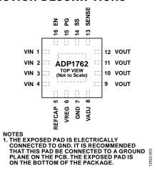
Figure 3. Pin Configuration
