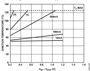
Figure 39. 25 mm<sup>2</sup> of PCB Copper,  $T_A = 50$ °C
