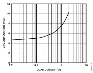
Figure 8. Ground Current vs. Load Current
