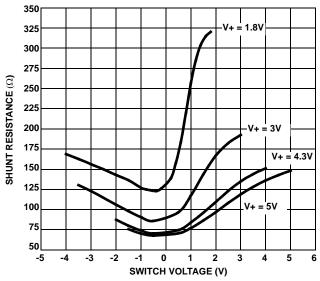
FIGURE 25. SHUNT RESISTANCE vs SWITCH VOLTAGE
