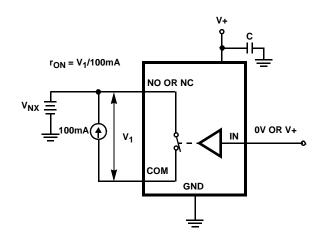
FIGURE 5. ron TEST CIRCUIT
