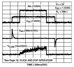
FIGURE 23. CLICK AND POP ELIMINATION  $20k\Omega$  LOAD 200ms DELAY
