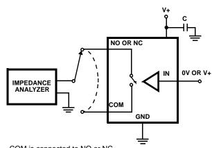
COM is connected to NO or NC during ON capacitance measurement.
