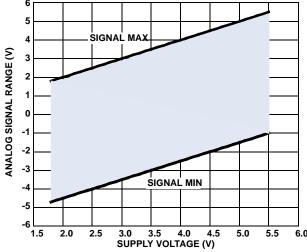
FIGURE 16. ANALOG SIGNAL RANGE vs SUPPLY VOLTAGE
