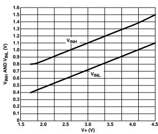
FIGURE 18. DIGITAL SWITCHING POINT vs SUPPLY VOLTAGE
