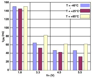
FIGURE 19. TURN - ON TIME vs SUPPLY VOLTAGE
