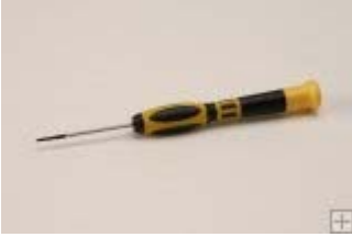
Phillips Screwdriver, #0 x 50mm
