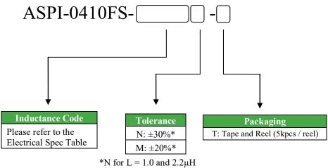
\*M for L = 1.0 and 2.2 $\mu$ H \*M for L = 2.2 ~ 47 $\mu$ H
