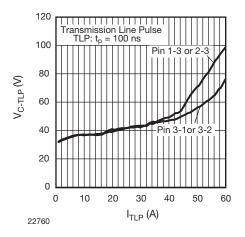
Fig. 6 - Typical Clamping Voltage  $V_{C\text{-}TLP}$  vs. Pulse Current  $I_{TLP}$
