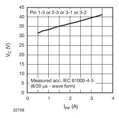
Fig. 5 - Typical Peak Clamping Voltage  $V_{\rm C}$  vs. Peak Pulse Current  $I_{\rm PP}$
